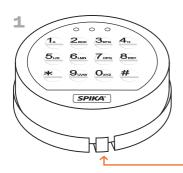
Press here while rotating digital lock face anti-clockwise.
